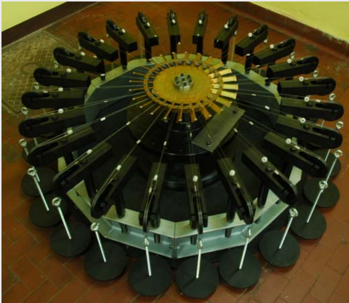
Non contact electromagnetic excitation
