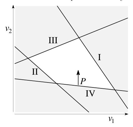
The four constraints exclude the (shaded) region of  $v_1v_2$ -space on one side of the lines I,II,III,IV respectively.
