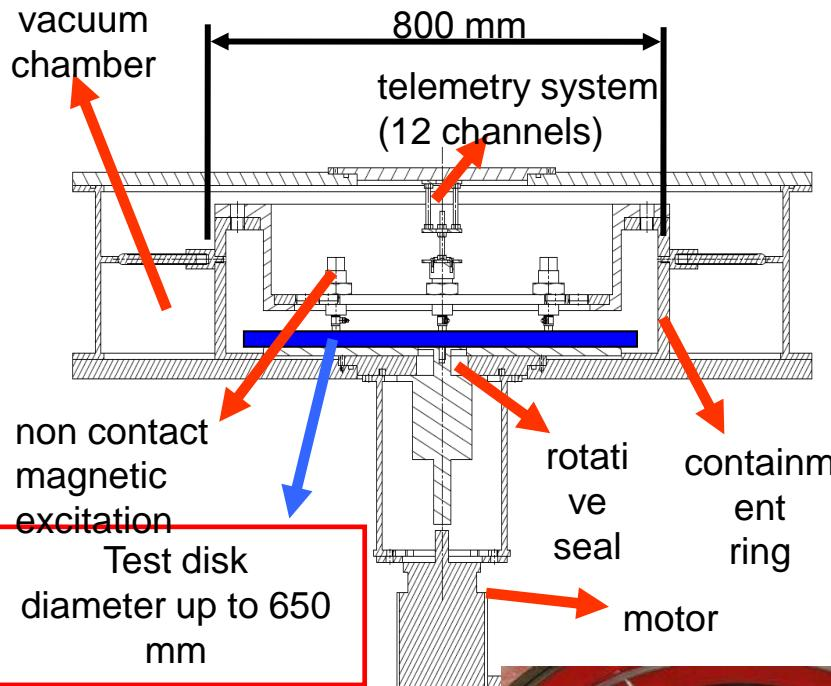
Rotation speed up to 4000 rpm
